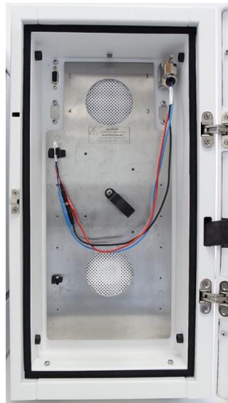
Figure 1. Opened oven compartment of the detector/potentiostat showing one external dummy cell installed (install more dummies in case of multiple board equipment). Make sure to fixate the dummy cell in a clip away from the fan as dangling will result in higher and out of spec noise levels.
